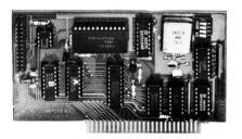
U-PORT is a single board having on it eight serial ports. These are RS232 type ports allowing both sending and receiving of data. Each port is, of course, individually addressable. The baud rates allowed, range from 150 to 19200. Three different rates may be simultaneously set up and then fed to eight ports grouped as 5, 2 and 1. All eight ports may be set to the same rate if required.
